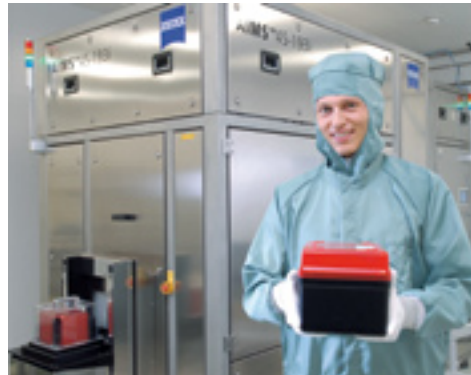
◀ The first: AIMS 45-193i is the world's first inspection system for checking masks in immersion lithography.
